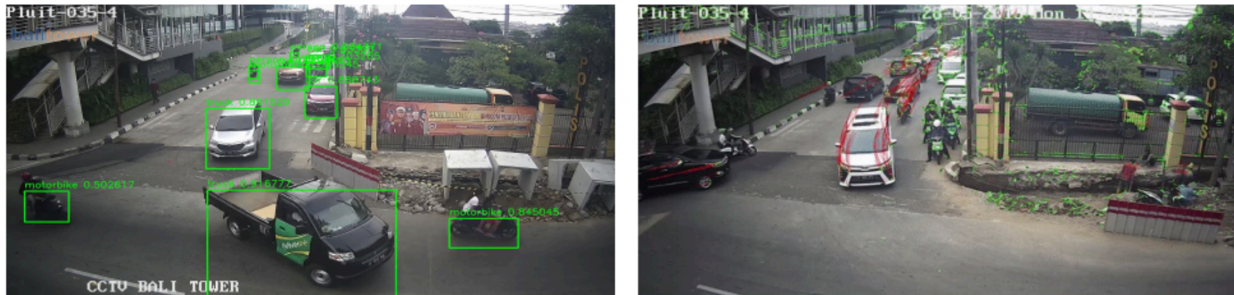
Figure 1: On the left, detection/classification with YOLOv3. On the right, motion detection with Lucas-Kanade Optical Flow.
