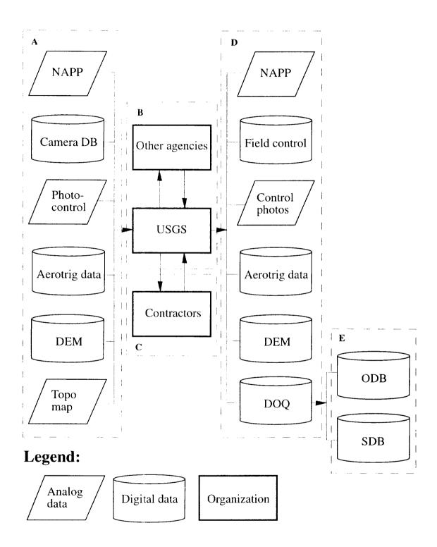
Figure 1. Digital orthophoto production system dataflow.
