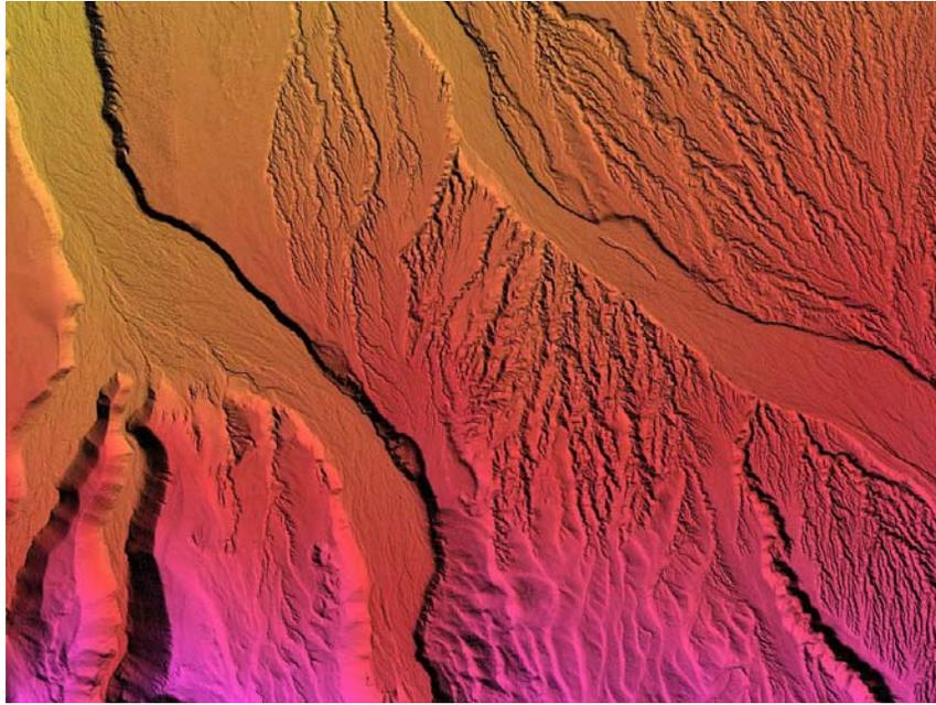
Figure2: 4m resolution DEM from digital aero-photos using multi-baselines, multiply matching features image matching algorithm. Up: urban area. Down: dry, semi-dry deep cutting broken area.
