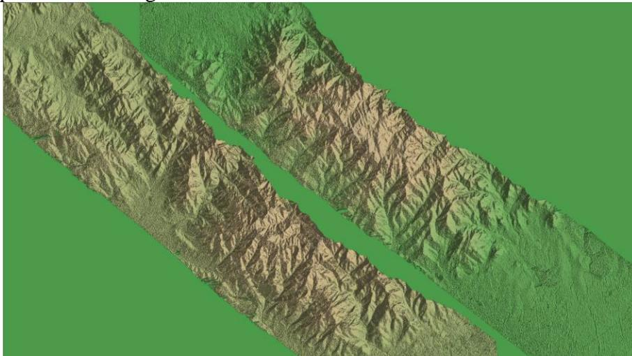
Figure 3: DEM from airborne double antenna SAR (airscape)
