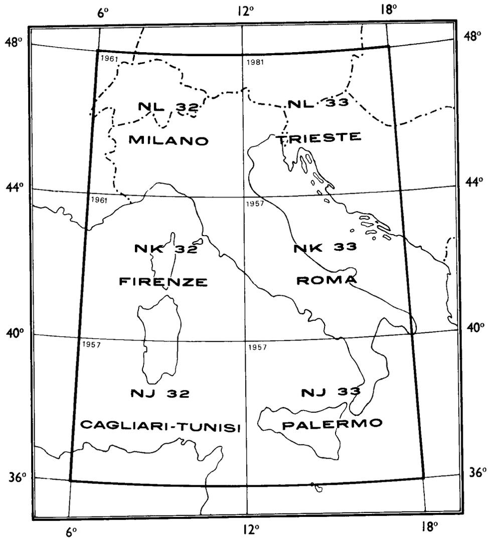
These sheets, released by the IGMI in a seven-colour version, have been produced according to the modified polyconic projection with the Clarke 1880 ellipsoid as the reference ellipsoid.
