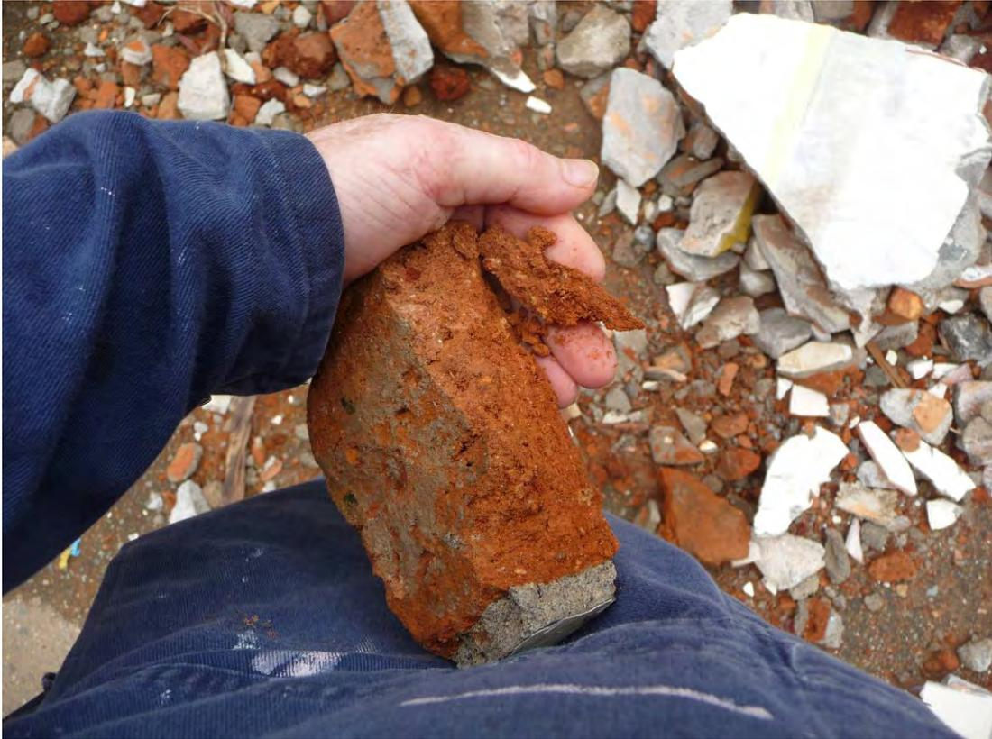
Figure 6 Soft bricks--Broken with fingers
