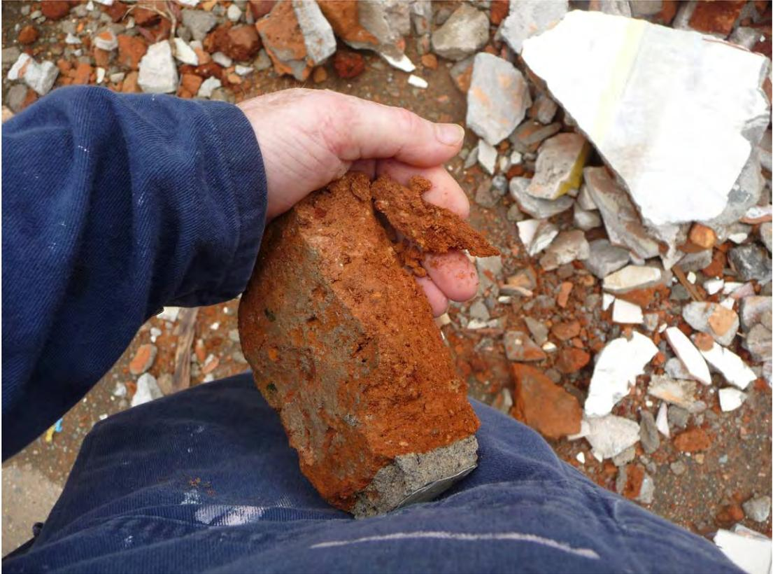
Figure 6 Soft bricks--Broken with fingers
