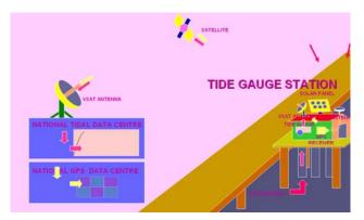
computational and communication infrastructure to enable reception of real-time data from all the sensors, analysis of the data, generation and dissemination of tsunami advisories.
