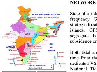
State-of-art digital tide gauges co-located with the dual frequency GPS receivers have been installed at strategic locations all along the Indian coastline and its islands. GPS receivers have been deployed to segregate the sea level rise from that of possible subsidence or upheaval of land mass.
