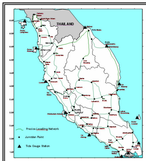
Figure 20: Precise Levelling Network (PLN)
