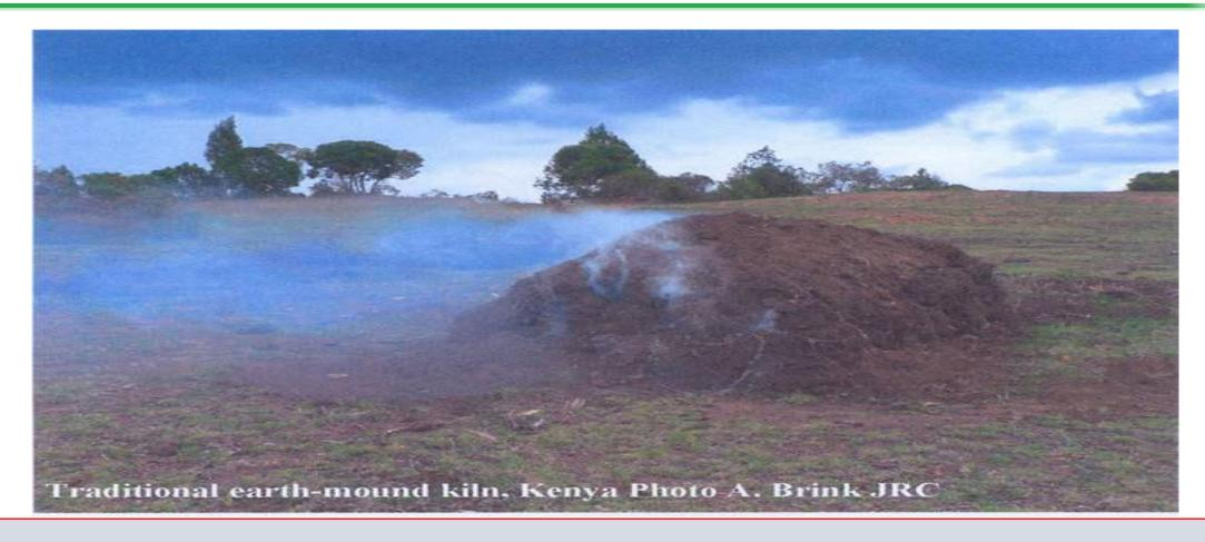
Using traditional kilns, 60-80% of wood's energy is lost in charcoal production process
