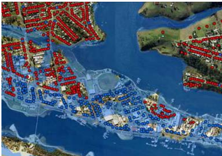
Figure 8. Sample result of combined modelling of a 1-in-100 year storm surge with a projected sea-level rise of 1.1 metre. Commercial (blue) and residential (red) buildings are from the NEXIS database.
