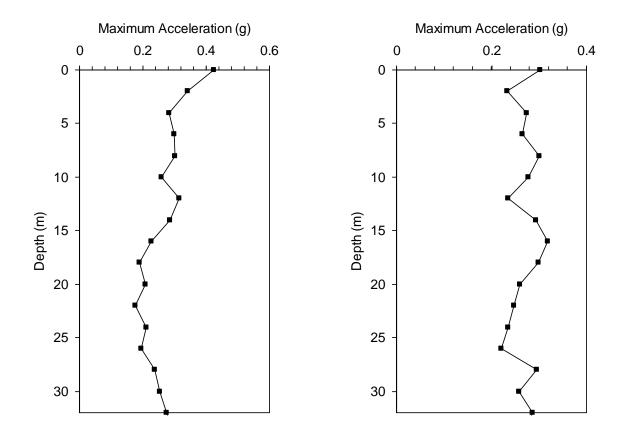
Figure 4.7. Variation of ground acceleration from base rock to the ground surface for soft and hard soil classification
