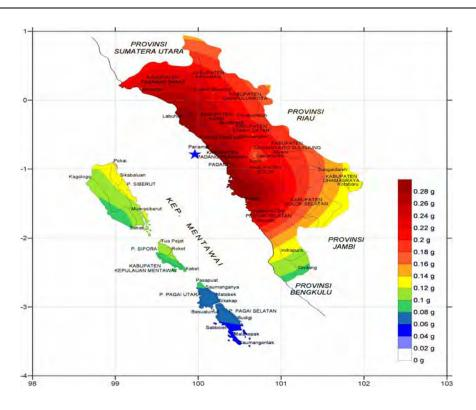
Figure 3.4 Estimated PGA (reference base-rock) spatial distribution using Young's Intraslab attenuation due to 30 September 2009 West Sumatra Earthquake
