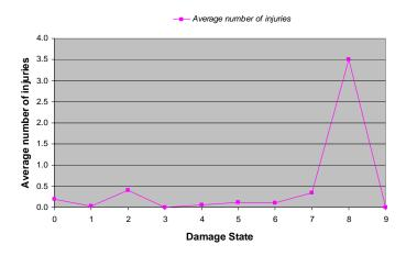
Figure 6.11: Average number of injuries per building versus damage state number.
