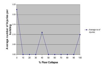
Figure 6.10: Average number of injuries per building versus percentage floor collapse.
