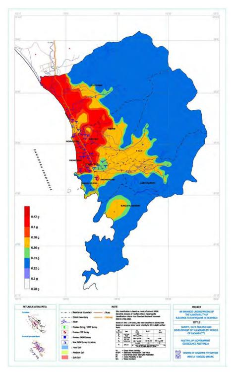
Figure 1. Spatial distribution of ground surface PGA for city of Padang
