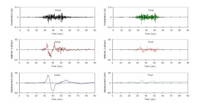
Figure 4.4. Scaled Input motion in corresponding to Spectral Matching, MASW26 (SD) (EZ-FRISK 7.32 Strong Motion Database)
