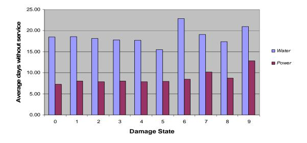
Figure 6.14: Average number of days without service plotted against building damage severity.
