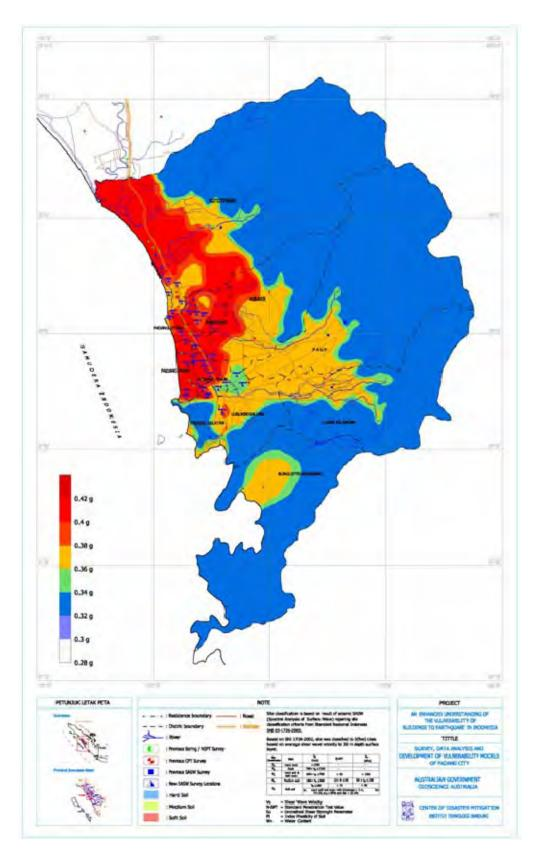
Figure 4.8. Peak Ground Acceleration (PGA) map for the city of Padang
