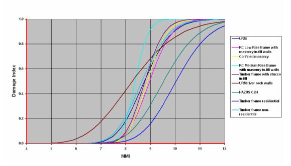
**Figure 7.2:** Workshop developed benchmark vulnerability curves derived from the Padang Earthquake damage observations.
