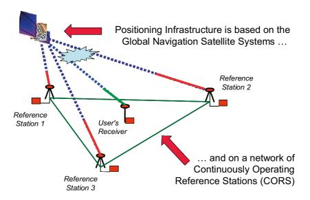
Figure 4.5: Components of a Positioning Infrastructure.
