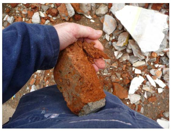
Figure 6 Soft bricks--Broken with fingers
