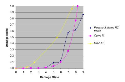
**Figure 6.2:** Damage index versus damage state number for the 3 storey office building. DI=0.000229\*2.76^(Damage State Number)
