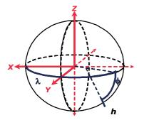
*Figure 4.6:* Mathematical model for a geodetic datum.
