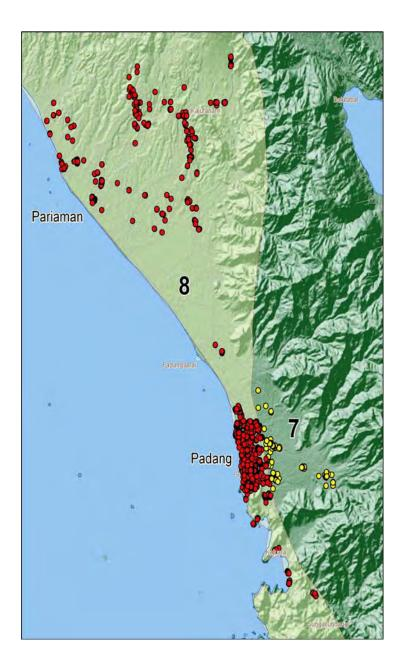
Figure 6.1: MMI attribution based on observed liquefaction, lateral spreading, landsliding and building damage along with resident interviews conducted by the survey team. Red dots show locations where an MMI of 8 was recorded. Yellow dots show locations where an MMI of 7 was recorded.
