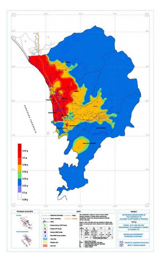
Figure 5.4: Spatial distribution of ground surface PGA for the city of Padang
