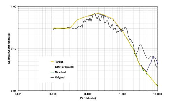
Figure 4.1. Spectral Matching, MASW23 (SE)
