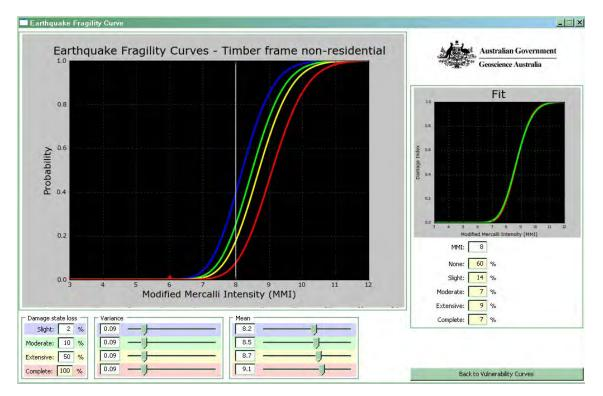
Figure 7.3: Screen view of Eloss fragility curve suite attribution software. Damage threshold curves are presented on the left graph based on heuristically selecting the median and variance values that collectively match the target damage state mix from Padang at MMI 8 (refer bottom right). The match of the curves to the previously adopted vulnerability curve is shown on the smaller graph to the right.
