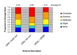
Figure 6.7: Consistency of fragility across different types of unreinforced masonry (URM) buildings
