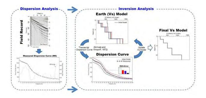
Figure 2.7. The inversion process to produce shear wave velocity profile
