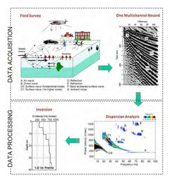
Figure 5.1: The overall procedure of Multi Channel Analysis of Surface Waves (MASW).
