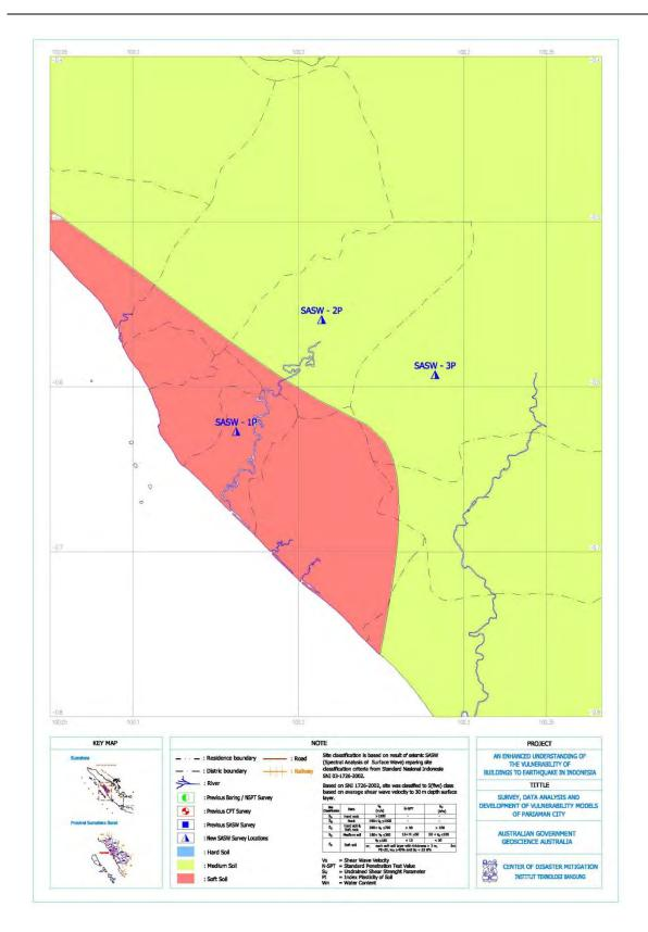
Figure 2.18. Combined Site classification map for city of Pariaman based on the recent MASW survey and previous geotechnical investigation
