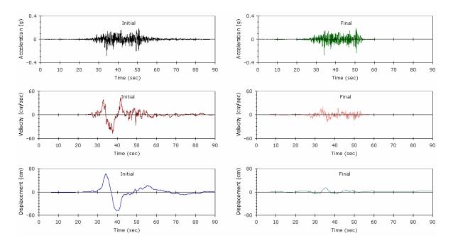
Figure 4.6. Scaled Input motion in corresponding to Spectral Matching, MASW28 (SC) (EZ-FRISK 7.32 Strong Motion Database)
