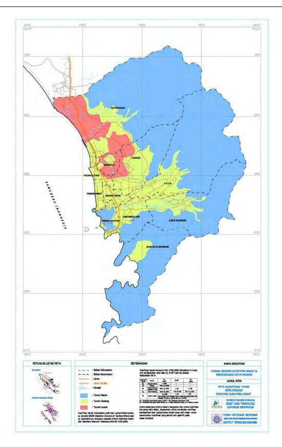
Figure 2.16. Site classification map for city of Padang based on the previous geotechnical investigation
