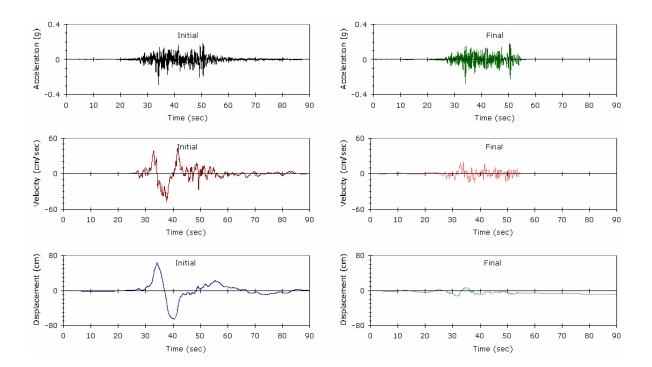
Figure 4.2. Scaled Input motion in corresponding to Spectral Matching, MASW23 (SE) (EZ-FRISK 7.32 Strong Motion Database)
