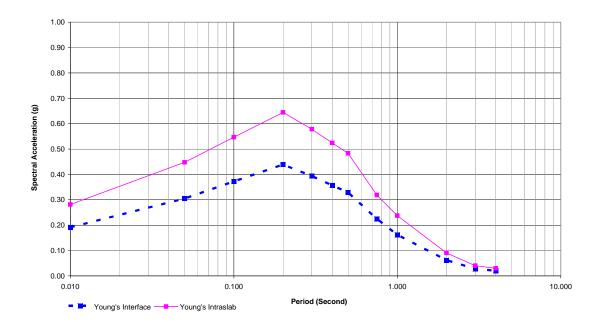
Figure 3.2. Deterministic baserock spectra result in Padang City developed using EZ-FRISK 7.32 Build 001
