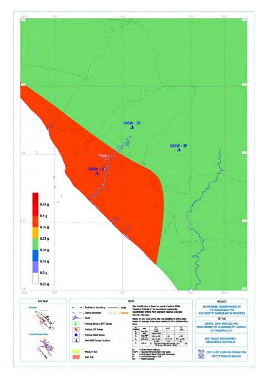
Figure 5.5: Spatial distribution of ground surface PGA for the city of Pariaman
