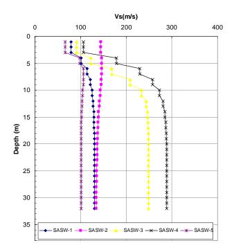
Figure 2.8. Shear wave velocity as function of depth of the MASW survey at point 01-05
