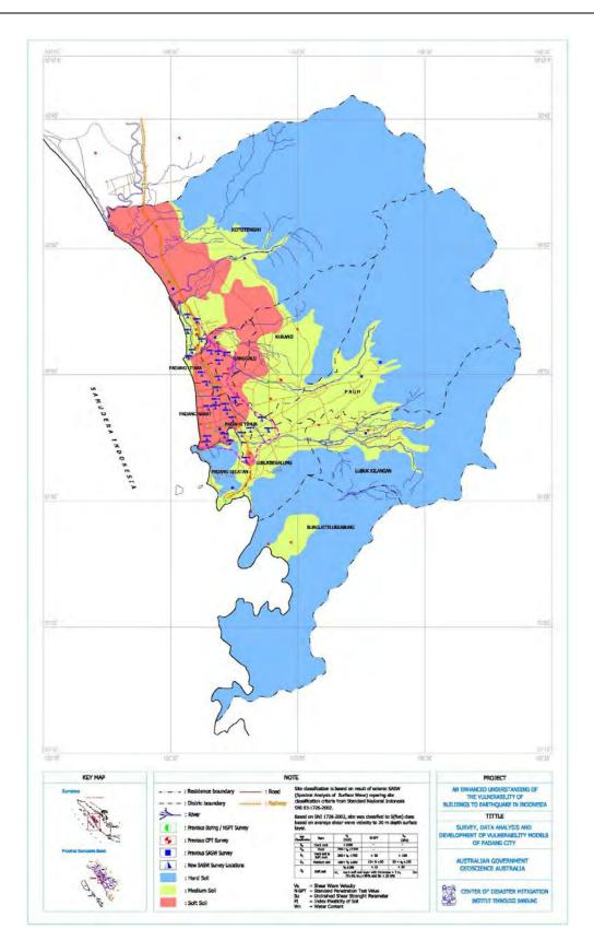
Figure 2.17. Combined Site classification map for city of Padang based on the recent MASW survey and previous geotechnical investigation
