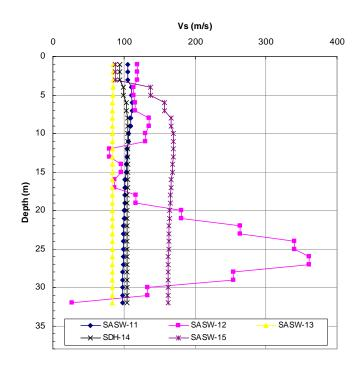
Figure 2.10. Shear wave velocity as function of depth of the MASW survey at point 11-15
