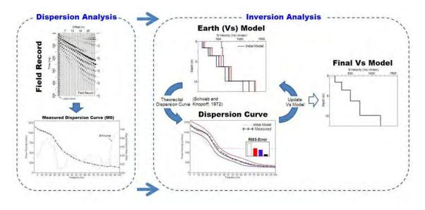
Figure 5.2: The inversion process to produce the shear wave velocity profile
