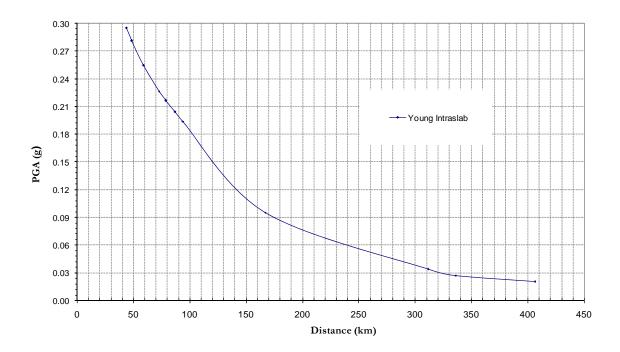
Figure 3.3. Attenuation curve of PGA (reference base-rock) of September 30, 2009 West Sumatra earthquake
