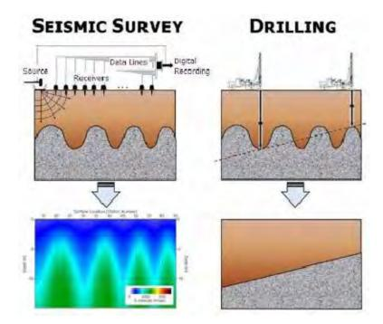
Figure 2.3. Comparison between the surface wave method and the drilling methods
