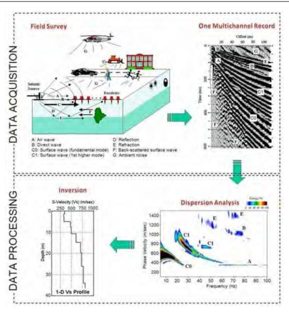
Figure 2.4. The overall procedure of Multi Channel Analysis of Surface Waves (MASW)
