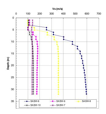
Figure 2.9. Shear wave velocity as function of depth of the MASW survey at point 06-10
