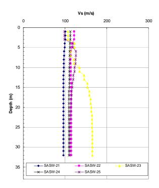
Figure 2.12. Shear wave velocity as function of depth of the MASW survey at point 21-25
