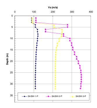
Figure 2.14. Shear wave velocity as function of depth of the MASW survey at point 1P-3P
