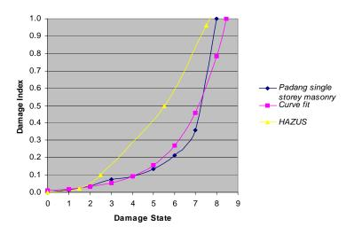
Figure 6.3: Damage index versus damage state number for the generic residential building. DI=0.0106\*1.72^(Damage State Number).
