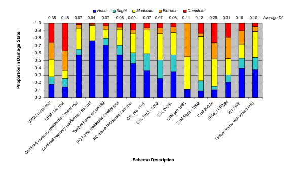
Figure 6.4: Fragilities for well represented building types in Padang subjected to MMI 8 shaking.
