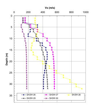
Figure 2.13. Shear wave velocity as function of depth of the MASW survey at point 26-30
