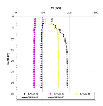
Figure 2.11. Shear wave velocity as function of depth of the MASW survey at point 16-20
