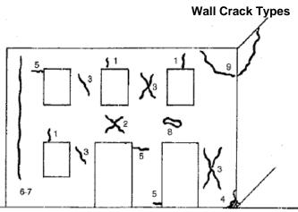
Figure 7: types of cracks in masonry bearing walls:
