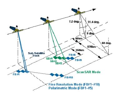
Fig. 4. PALSAR observation geometry for each mode
