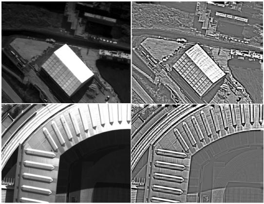
Figure 1: Left column: Original aero-photos after image contrast stretching; Right column: Aero-photos after adaptive image edge enhancement.
