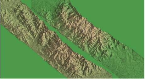
Figure 3: DEM from airborne double antenna SAR (airscape)
