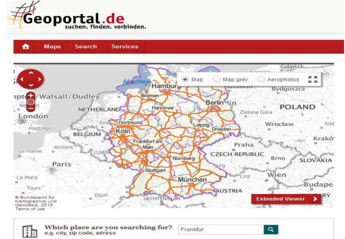
The German national geographical names database (GN-DE) published as a web service as part of the national spatial data infrastructure (GDI-DE) and visualized through the Geoportal application (Geoportal.de)
