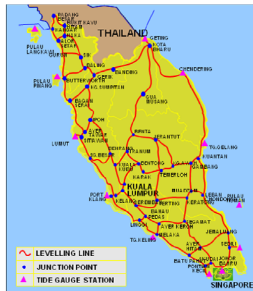
Figure 3 – Precise Leveling Network
