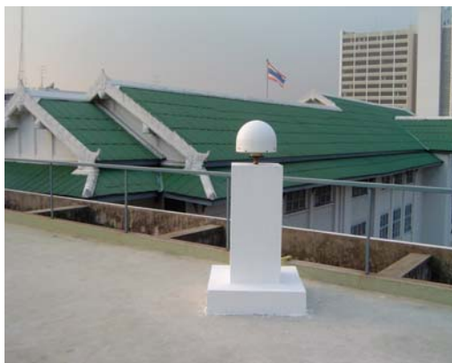
Fig. 6 RTSD-DEOS GPS permanent station at Survey School, RTSD
