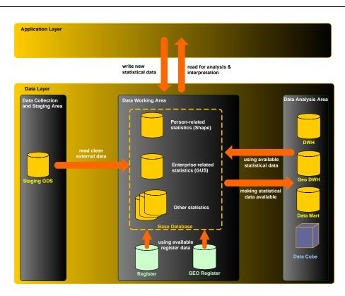
Figure 5 – Data flow in the data working area
