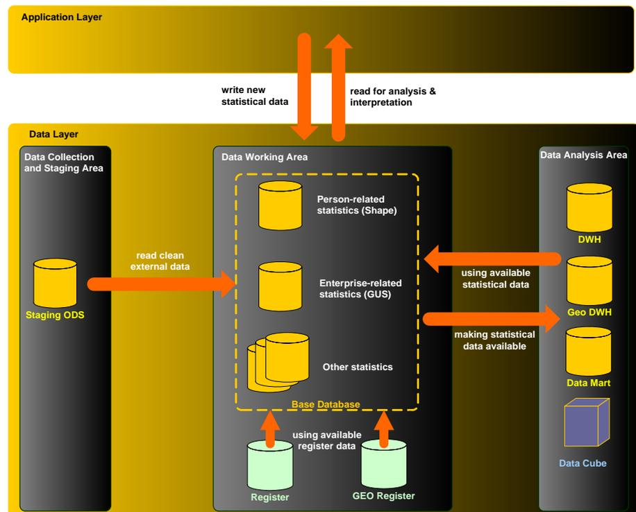
Figure 5 – Data flow in the data working area
