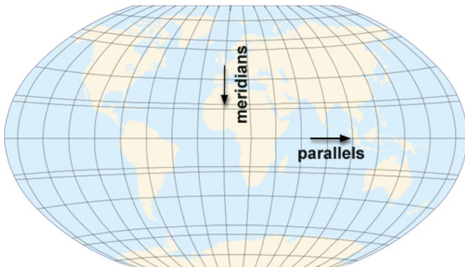
Latitude of a place on the globe, is measured north or south from the equator as angles, in degrees, minutes and seconds. Longitude is similarly measured as an angle east or west from the prime meridian of Greenwich, England. These measurements thus constitute a precise quantitative system.
